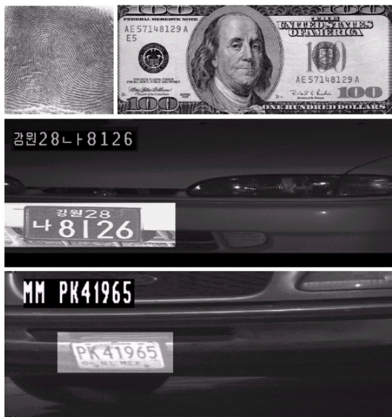
FIGURE Some additional examples of imaging in the visual spectrum. (a) Thumb print. (b) Paper currency. (c) and (d). Automated license plate reading. (Figure (a) courtesy of the National Institute of Standards and Technology. Figures (c) and (d) courtesy of Dr. Juan Herrera, Perceptics Corporation.)
